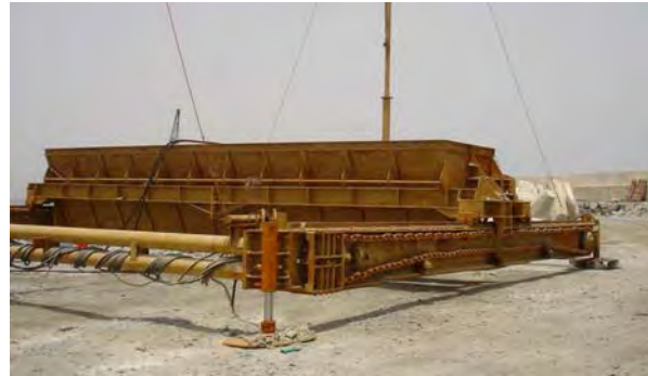
Figure 4—Traveling Screed Hopper (Khor Fakkan)
