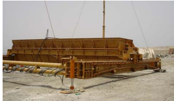
Figure 4—Traveling Screed Hopper (Khor Fakkan)
