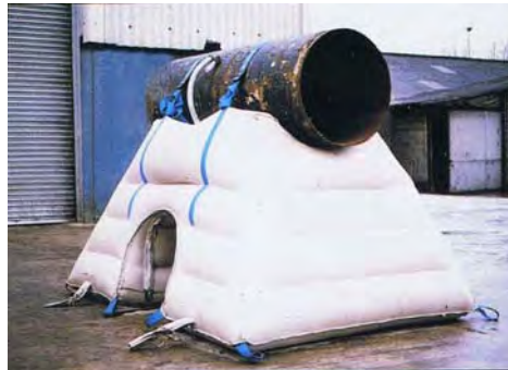
Pipe Support Block Test
